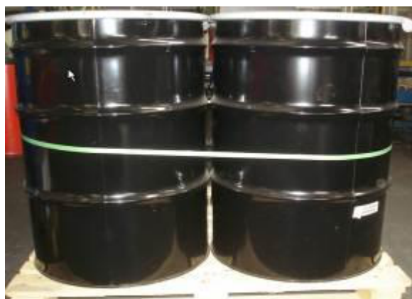
Good transportation securing (figure 1)
