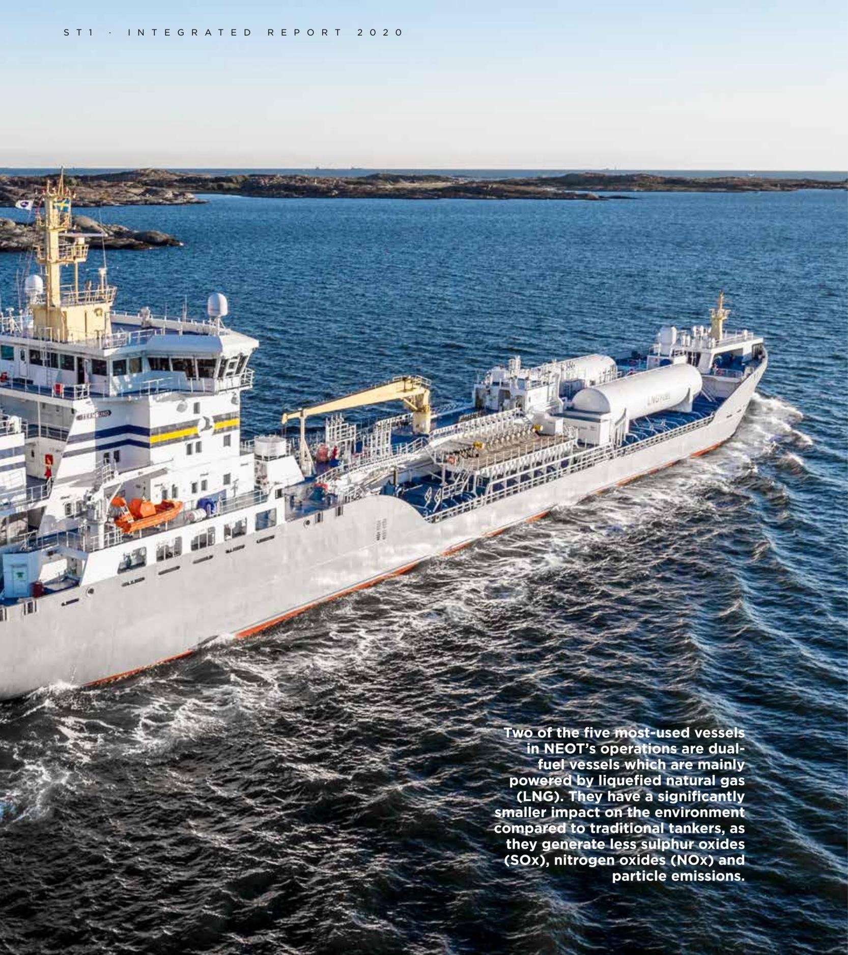
**Two of the five most-used vessels in NEOT's operations are dual-fuel vessels which are mainly powered by liquefied natural gas (LNG). They have a significantly smaller impact on the environment compared to traditional tankers, as they generate less sulphur oxides (SOx), nitrogen oxides (NOx) and particle emissions.**
