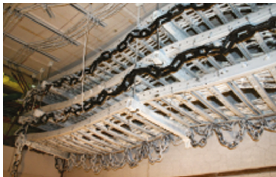
Test setup with cable ladders after the 90-minute fire test
