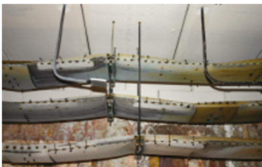
Test setup with cable trays after the 90-minute fire test
