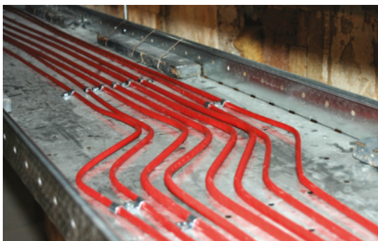
Test setup with cables in mandatory S-bend configuration
