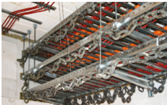
Test setup with cable ladders
