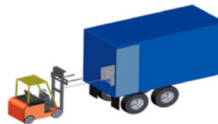
Figure 1d Incorrect method (using a pulling chain) of removal from a container
