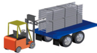
Figure 1b Incorrect method of removal
