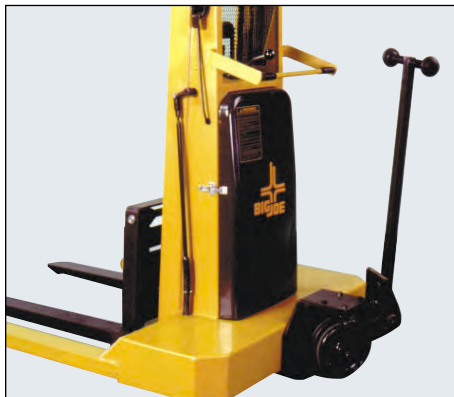
Steer Wheel The steer wheel configuration reduces steering effort and rolling resistance. This system improves maneuverability while making operation easier. Available for all models. The attachment consists of dual 8" x 2" phenolic resin wheels and spring loaded "T" bar handle for maneuvering with rated loads. Not available on R6 or R7 models.
