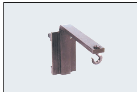
Boom with Hook Converts lift truck for portable crane operation. 26" long, 300 lb. capacity (500 lb. with proper straddles).
