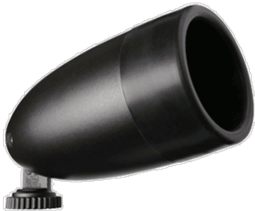
Premium PAR38 Flood with large, molded high temperature black silicone gasket that totally seals lamp. Die cast aluminum housing. EZ Locknut. Suitable for mounting within 4' of the ground. PAR38 or PAR20, 150 Watt max. Lamp not supplied. Color: Silver gray Weight: 0.8 lbs
