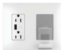
radiant® Wireless Charger with 15A Tamper-Resistant USB Type-A Outlet 5W Qi wireless charging pad; 3.1A charging capacity for Type-A port.
