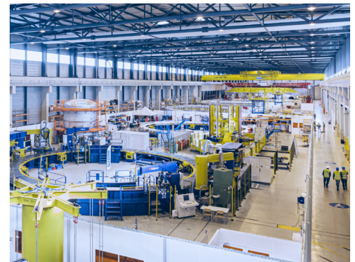
View of ITER Poloidal Field coils factory on-site, where four of the five coils that Europe is responsible for will be manufactured. © F4E
