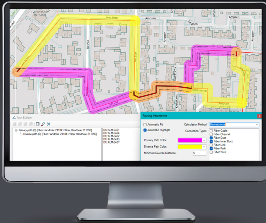
The primary path, diverse path and SPOFs are displayed in NetWorks Comms | Route Analyzer.
