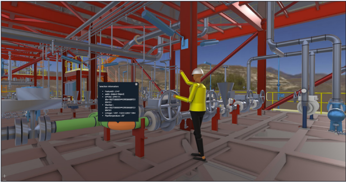
Figure 8: Monitor editable building information through selection and expression-based styling on 3D data.
