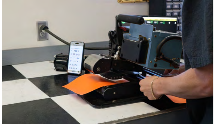
fig 9 | This is an example of a wedge welder.
