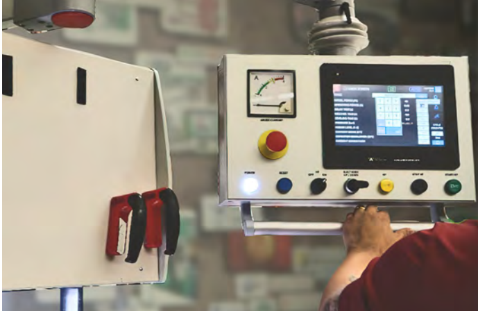
fig 12 | An example of a control panel for an RF welder.
